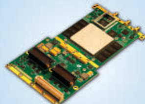
XPedite2400 Xilinx Virtex-7 FPGA-based XMC with high-throughput DAC
