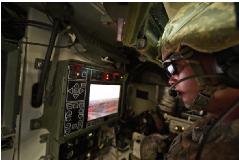
Engineers have integrated Lync, enabling warfighters in vehicles to exchange messages and share a common operating picture of the battlefield. (Image courtesy U.S. Army.)
